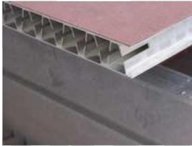
Fig. 2.8 Lateral milling to fit a T-shaped profile.
