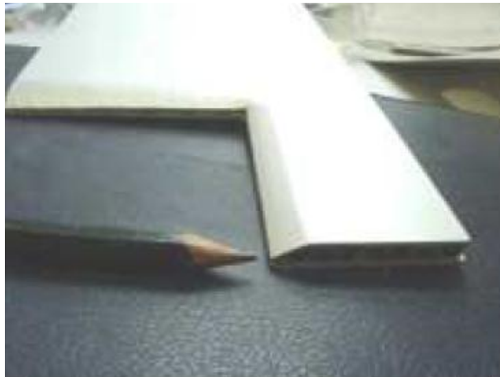
Fig. 2.7 Detail of wall panel cut with hydraulic corner notcher.
