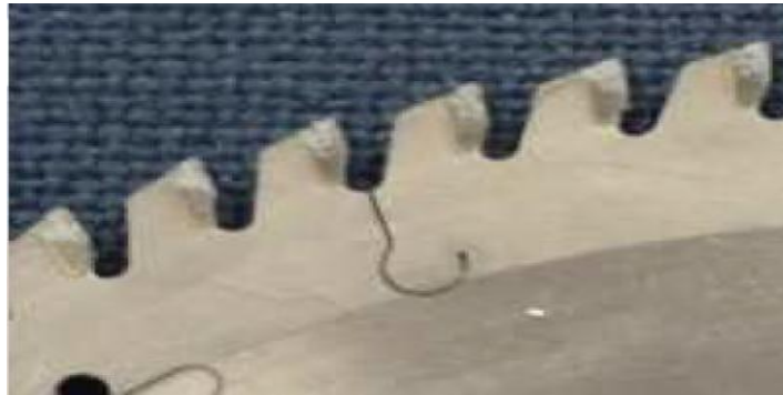
Fig.2.5 Saw for aluminium diam. 250 mm, bore 32 mm; 72 teeth; max rpm: 8000; recommended rpm: 3800.
