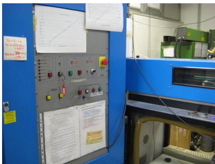
Figure 5.6: Laser control panel.
