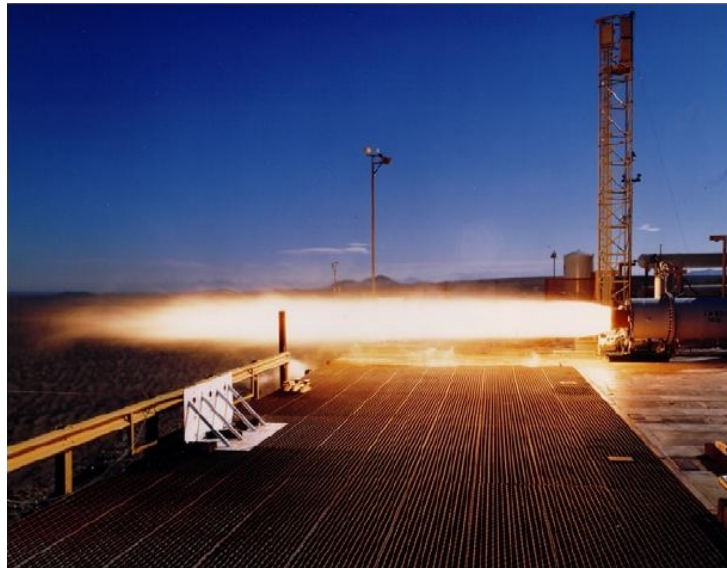
Figure 2.2: A 312 kN Hybrid rocket motor tested by AMROC.
