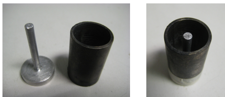
Figure 4.2: Central bone and cylinder (left), mould ready for the casting (right).
