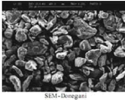
Figure 3.5: SEM image of tested magnesium hydride. Particles exhibit irregular shape [21].
