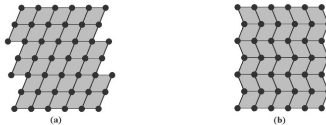
Figure 1.6 - The two mechanism of accommodation: (a) slip, (b) twinning
