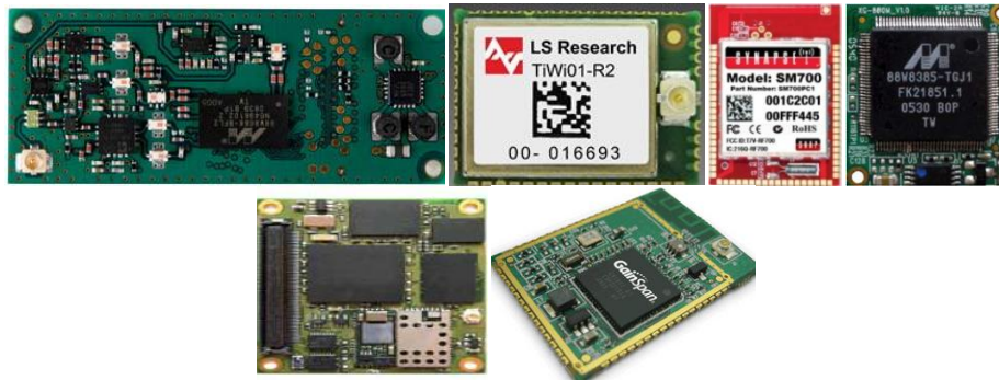
Figure 2.3 – IEEE802.11b ISL transceiver, from the left to the right: WiBear[37], TiWi-R2[38], SM700PC1[39], XG880MU[40], HW86052[41], GS1011M[42].
