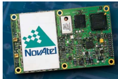
Figure 4.6 - NovAtel OEM4-G2L hardware
