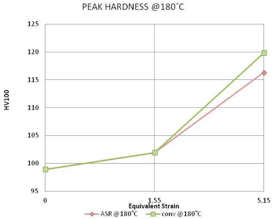
Fig. 5.18 Peak Hardness as a function of equivalent strain (Conv & ASR) at the aging temperature of 180°C
