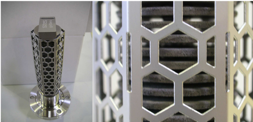
Figure 77 – NEG cartridge used as H 2 source for transmission tests along the CMS vacuum sector.
