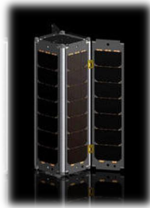
Figure 9.1. Double deployed panels for a 3U structure [26]
