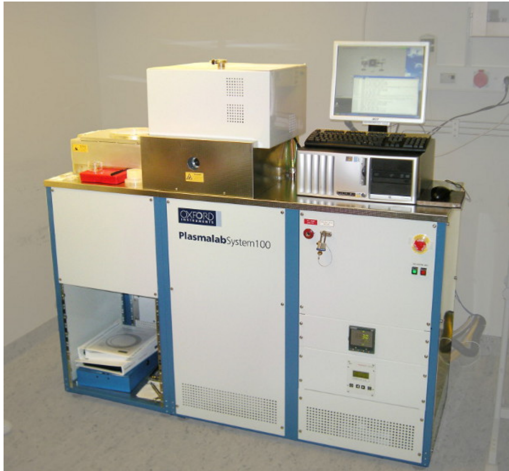
Figure 3.11: Plasmalab System 100 RIE machine by Oxford Instruments in the Nano Fabrications Lab at the Applied Physics department at KTH.
