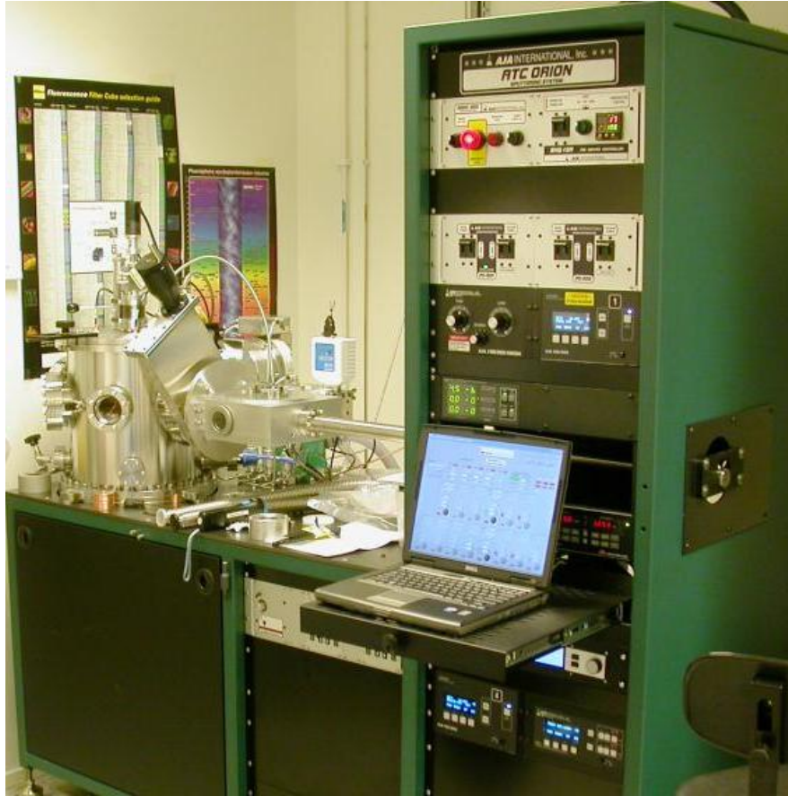
Figure 3.1: AJA Orion Sputtering System in the Nano Fabrications Lab at the Applied Physics department at KTH.
