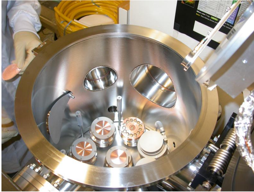
Figure 3.2: Main chamber of the AJA Orion Sputtering System. We can see the circular geometry in which the sputtering guns are positioned inside the chamber.
