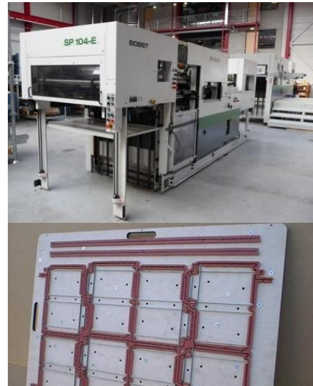
Figure 14 Die Cutting machine on the top and a Die on the bottom
