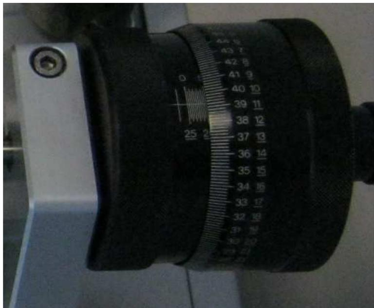
**Figure 4.8 Micrometric head**
