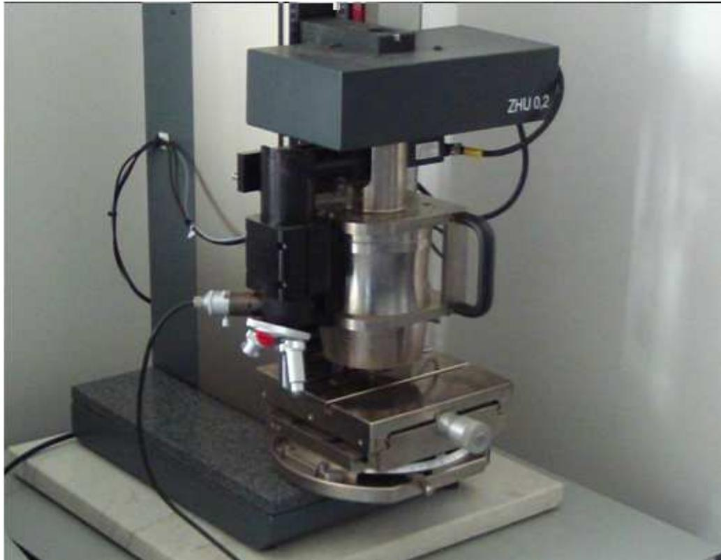
**Figure 6.32 Durometer Zwick ZHU 0.2**
