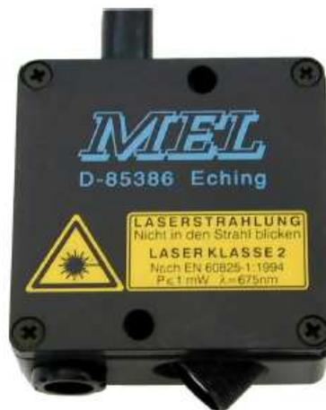
Figure 4. 10 Laser displacement
