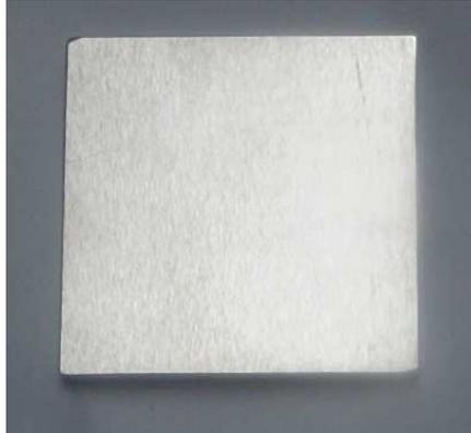
**Figure 3.6 Sample too reflective after grinding**
