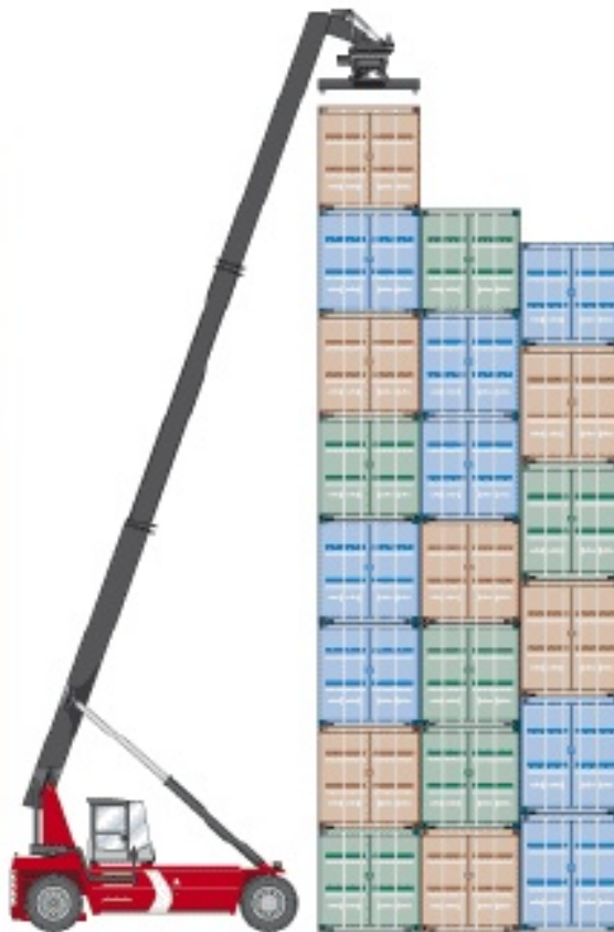
Figure 10 – A Reach Stacker grabbing a single container
