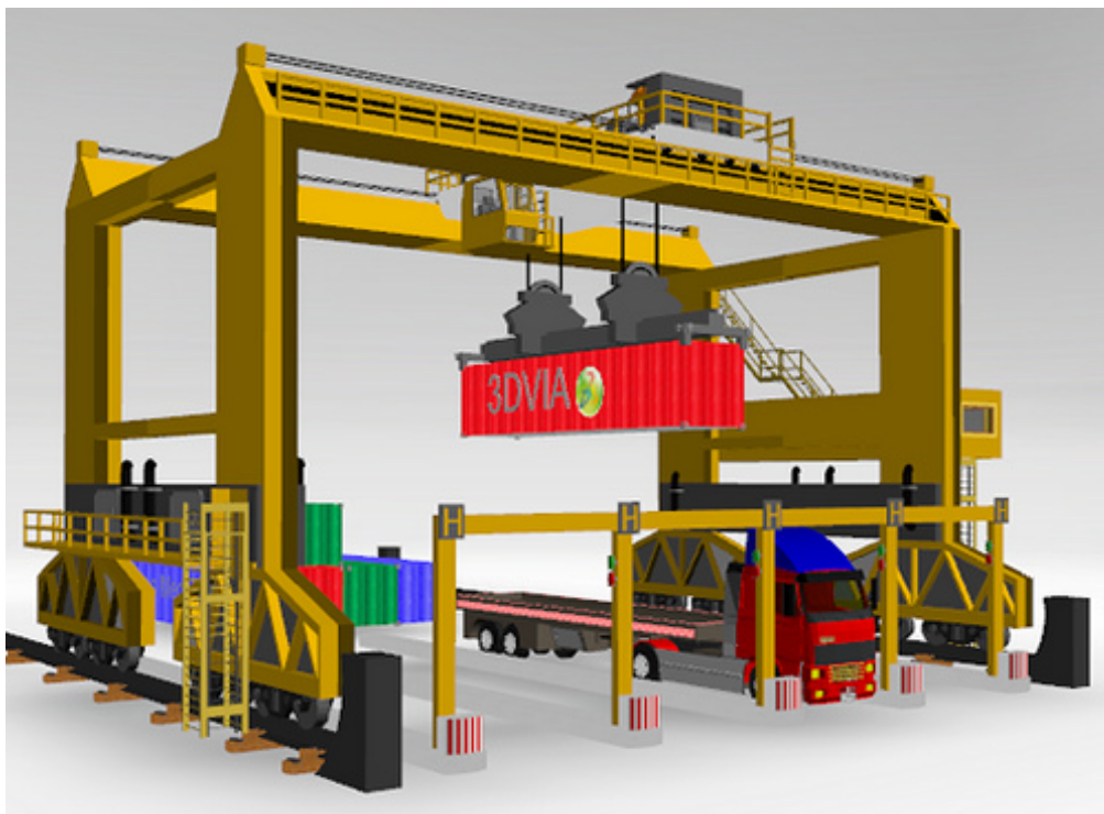
Figure 8 - The 3D model of a Liebherr RMG crane
