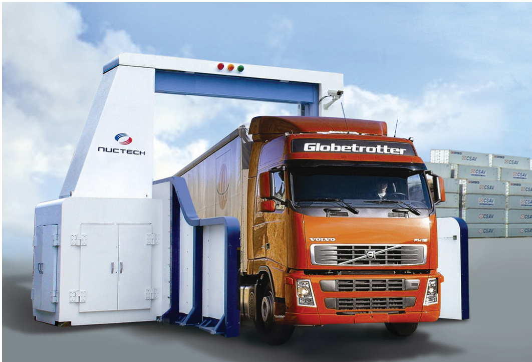
Figure 21 - An example of an x-ray terminal station
