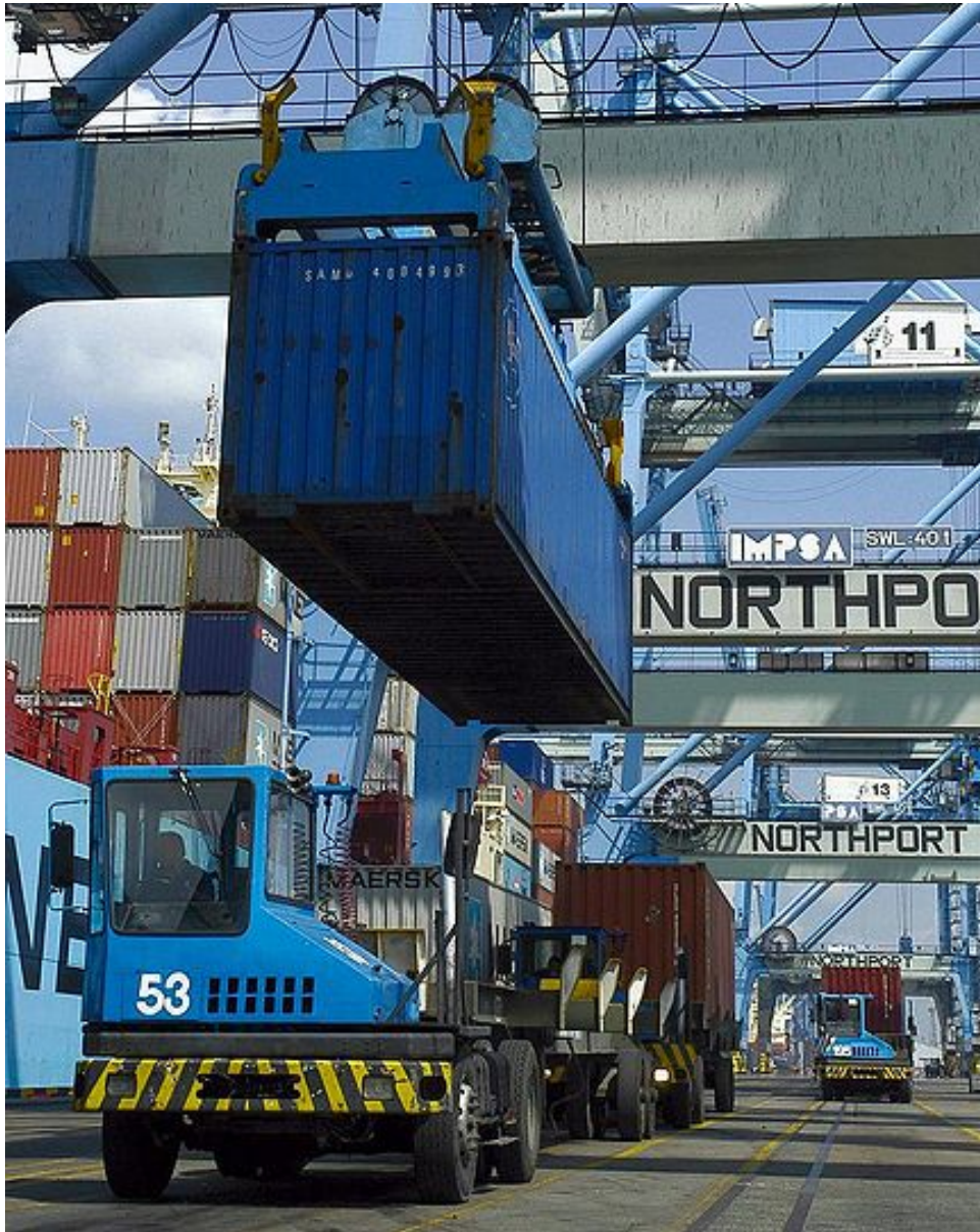
Figure 14 - A prime mover during yard operation
