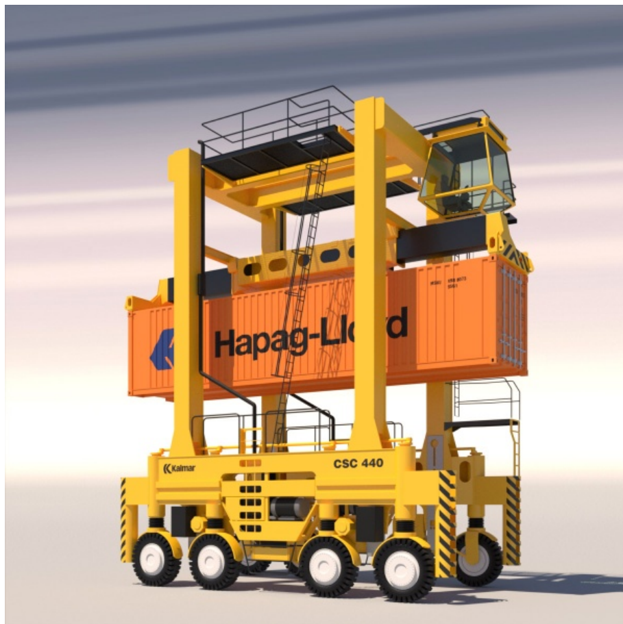
Figure 12 – A 3D model of a straddle carrier
