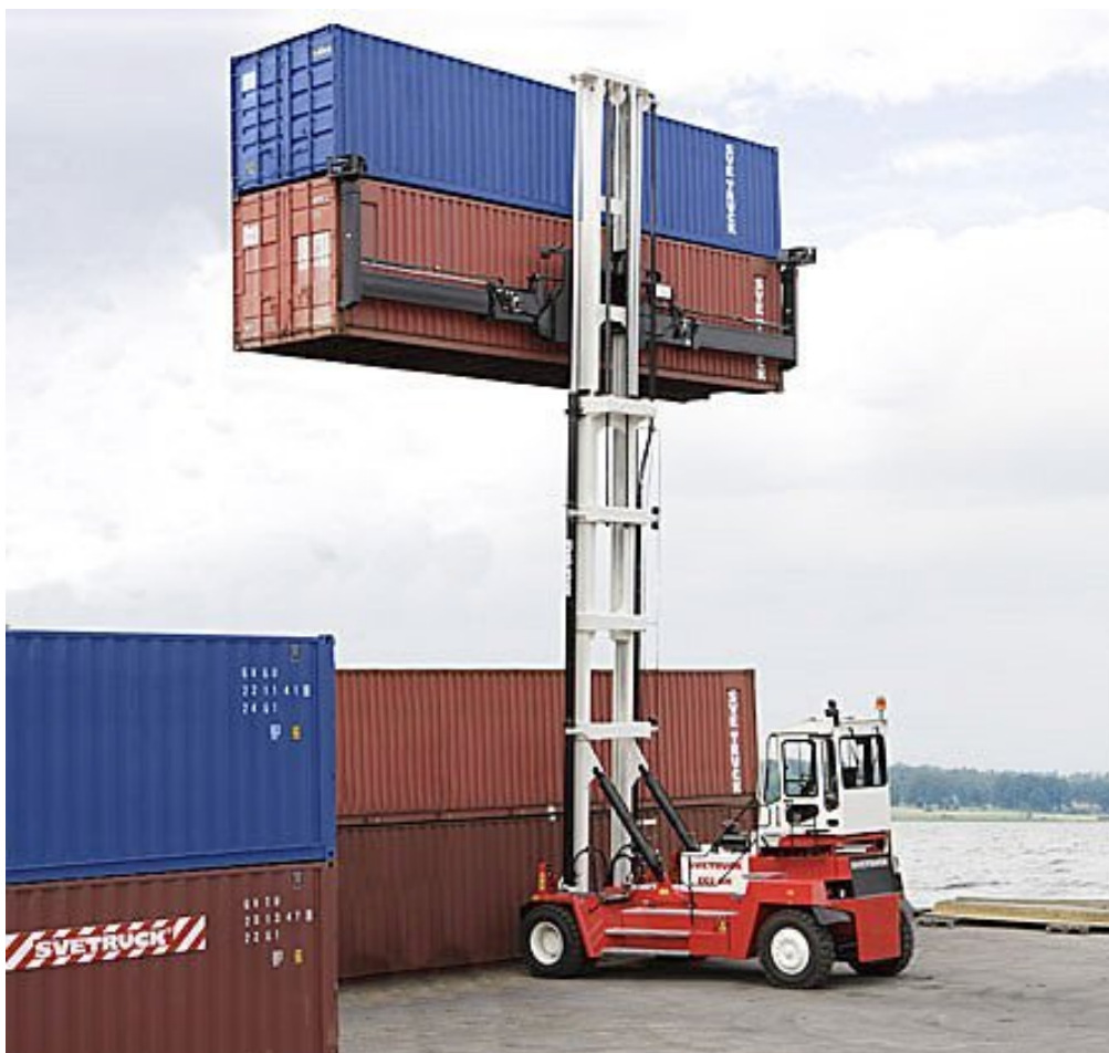
Figure 11 – A forklift truck handling with side-lift spreader
