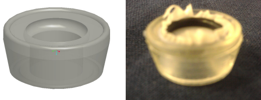
Figure 5: Modified cartridge, without o-ring in CAD model (left) and with the o-ring constraining the BAM (right).
