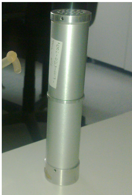
Figure 2.2: Test object used to verify the device's calibration.
