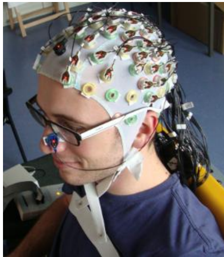
Figure 1.2: Cap with 62 electrodes positioned over the author's scalp for an EEG experiment.
