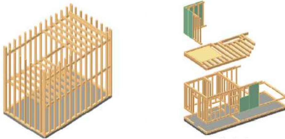
Fig. 2.21-2.22 Balloon Frame e Platform Frame
