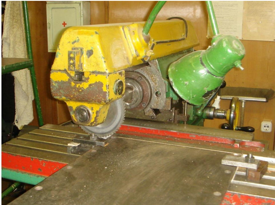
Figure 3.4: cutting of the stripes with a sawing machine
