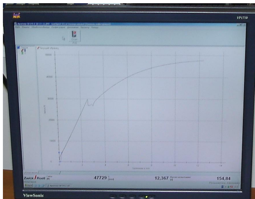
Figure 3.11: graph force-displacement. It is automatically drawn by the “testXpert®” software in real time during the experiment and it allows to save the data.
