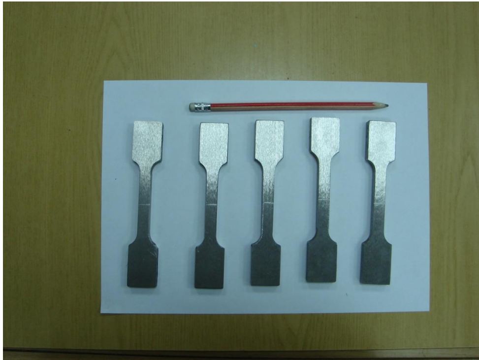
Figure 3.9: specimens at the end of manufacturing process. It is possible to note the little incision on the surface, realized to induce the breaking in the middle of the specimens.
