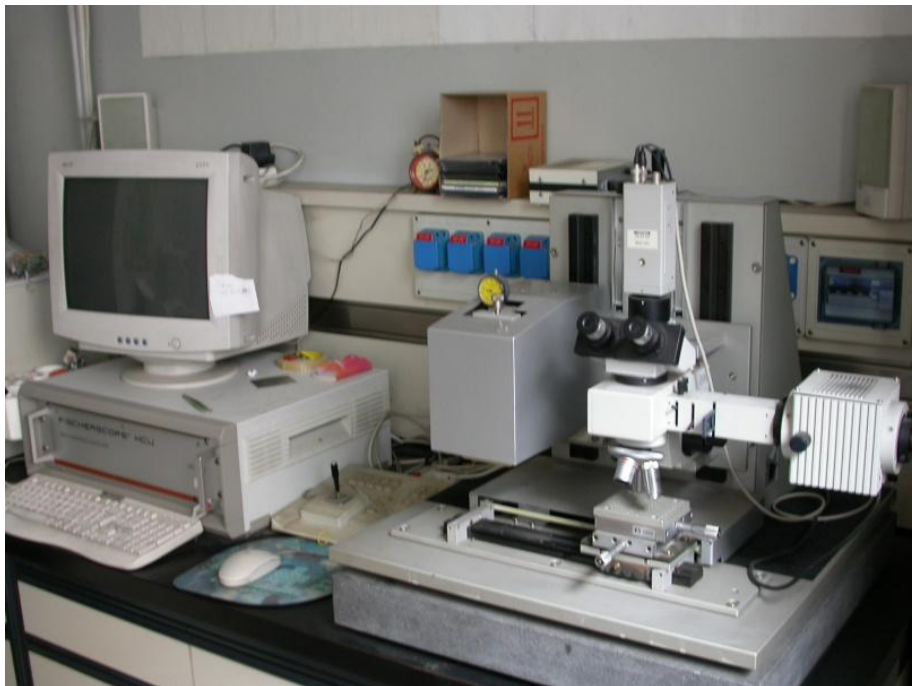
Figure 24: Vickers Microindentation Instrument.
