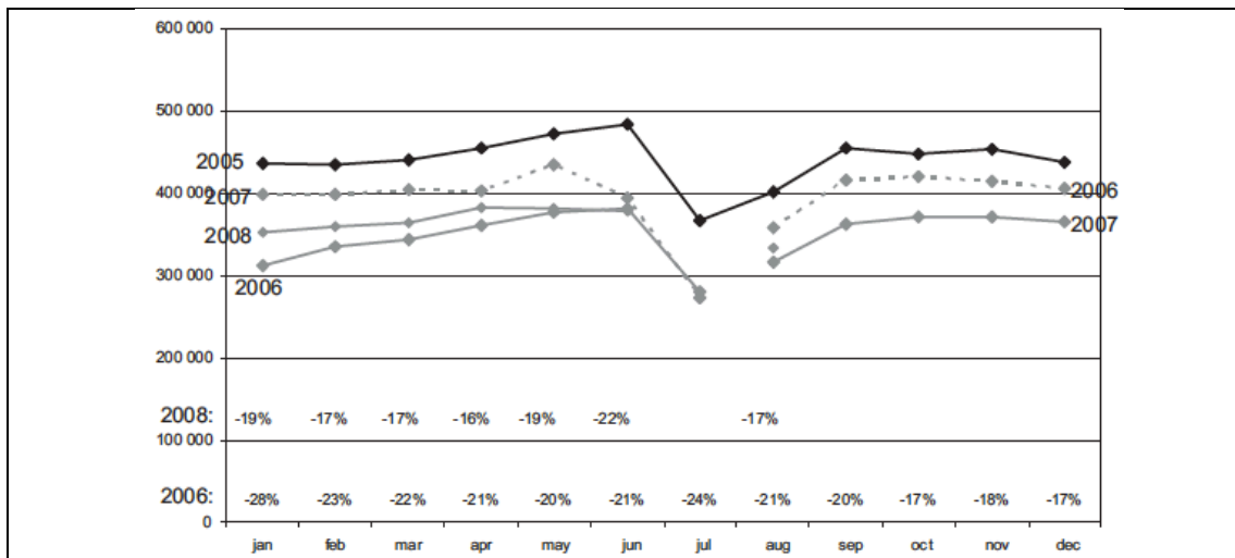
Figure 38. Number of vehicles across the cordon during charged hours, 2005-2008. Dashed lines indicate the time periods between the end of the trial and the reintroduction. The percentages at the bottom are traffic decreases relative to 2005 (Source: Eliasson, 2008, p.399)
