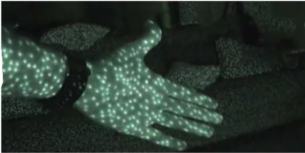
Figure 9: structured light pattern generated by the Kinect infrared laser projector.
