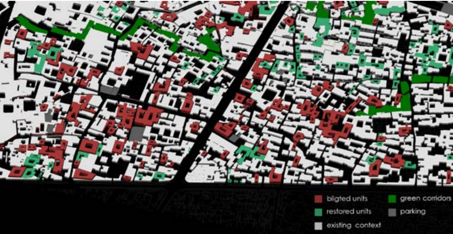
64 According to scenario 4, potential redevelopable plots in a buffer of 100 meters to the urban axe are targeted for renovation to provide a network of mixed active uses. The sketch presents plots targeted for renovation (adaptive reuse-change of density) in red and plots intended for conservation (improvement and preservation) in green.
