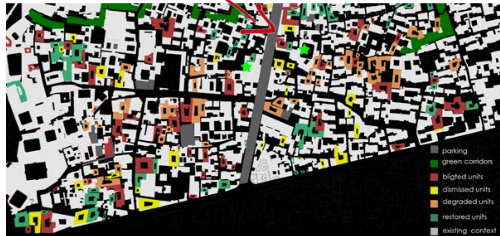
63 The scheme above shows existing situation. The sketch below depicts potential plots for redevelopment. According to scenario 4: blighted, dismissed and 68% of the degraded potential plots would be renovated as a network of mixed used (commercial, office, residential plots), 32 percent of the degraded plots would be conserved and improved (source:author's drawings)
