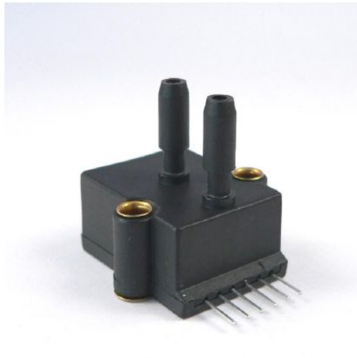
Figure 2.3: The pressure sensor used during the experiments
