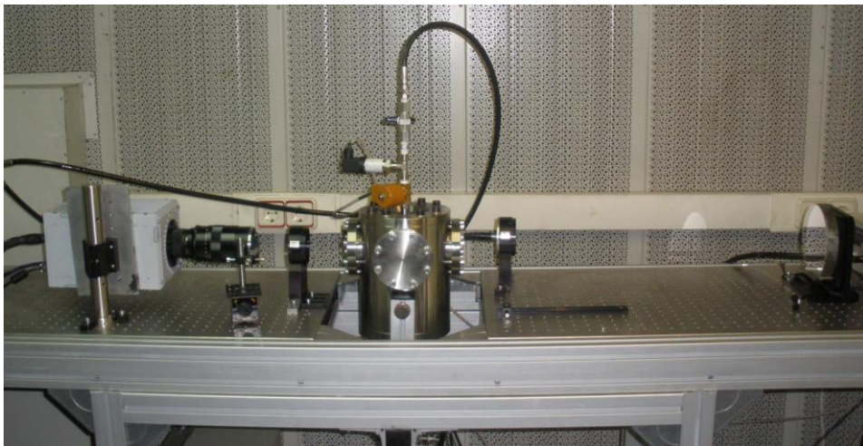
Figure 54: Real arrangement for testing with high speed camera
