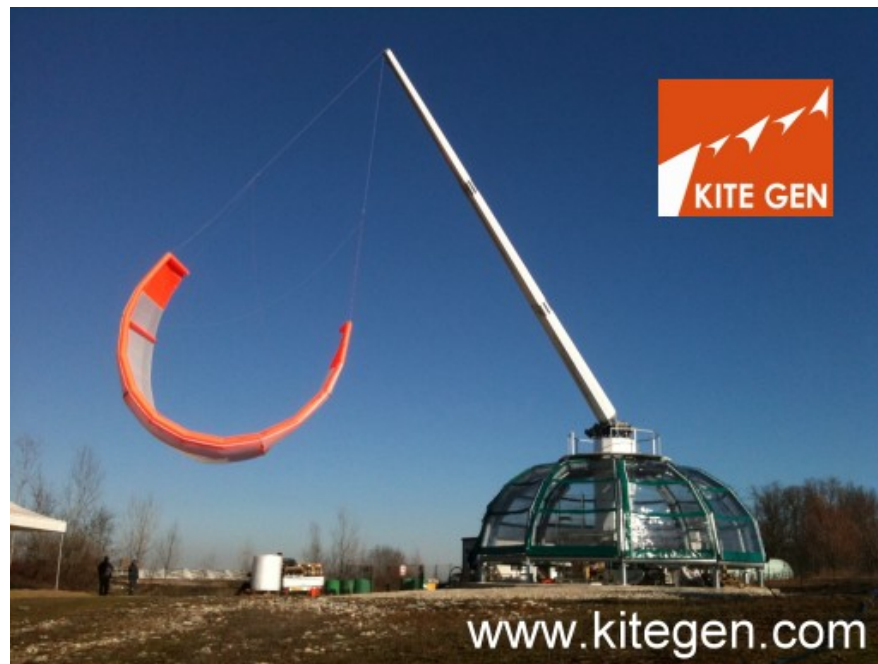
Figure 4.4: Kitegen Stem - 3 MW power plant, located in Sommariva Perno (CN), Italy. Picture from (22).
