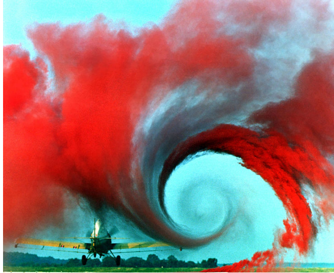
Figure 6.6: Vortex pattern generated by the passage of an aircraft - Picture from NASA in public domain.
