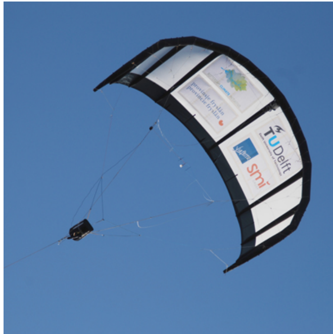
Figure 4.10: TU Delft kite - 25 m 2 leading edge inflatable kite with suspended, tele-operated control unit. It can reach 70 - 90 km/h generating a force of about 4000 N. Picture from (27)
