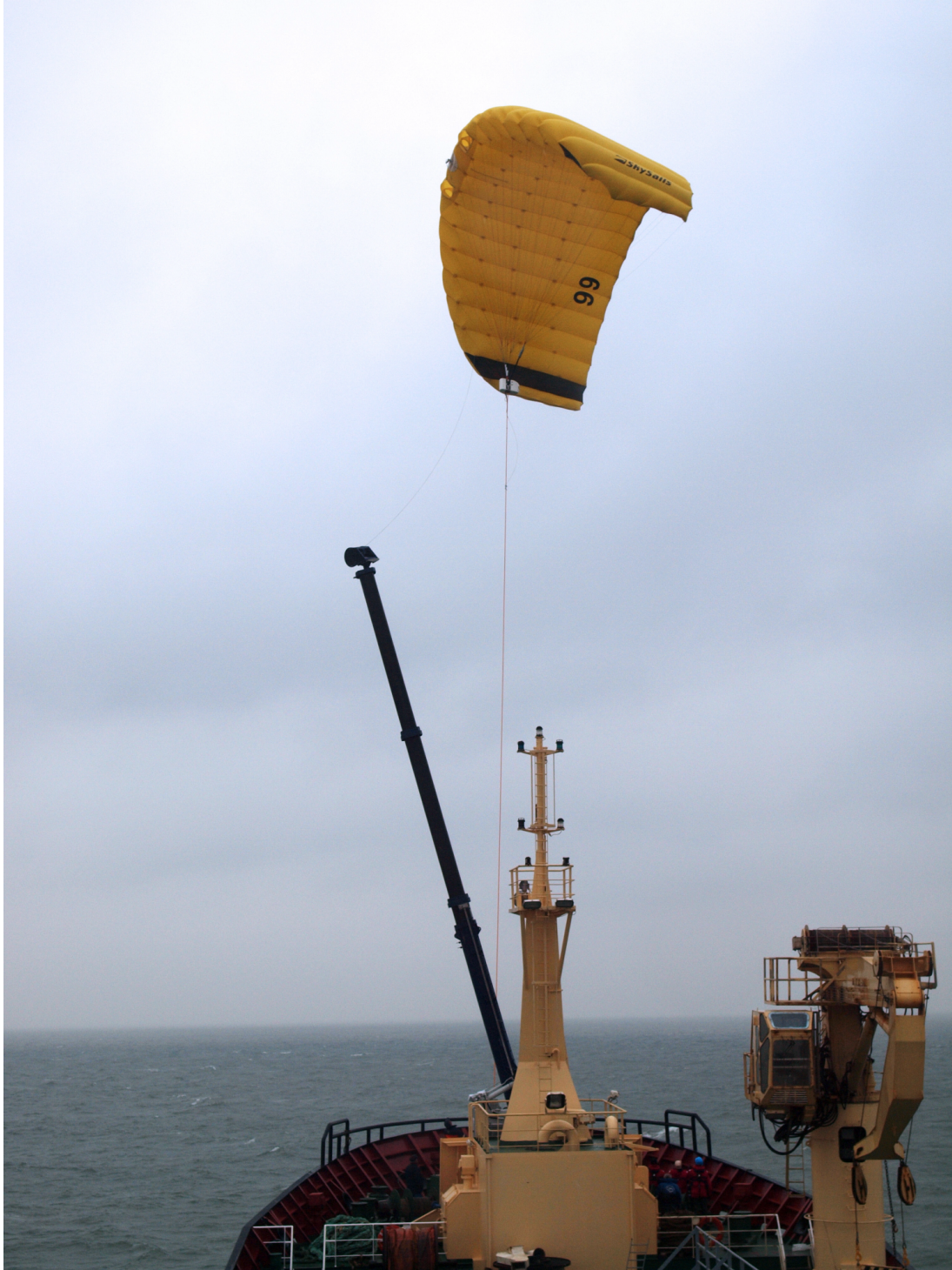
Figure 3.2: Skysails ram air kite - A ram air kite towing the ROS-171 'Maartje Theadora'. Picture from (12).
