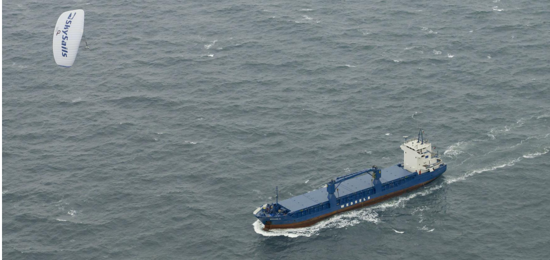
Figure 4.8: Skysails kite towing system - Kite towing the ship with only one cable. Picture from (12).
