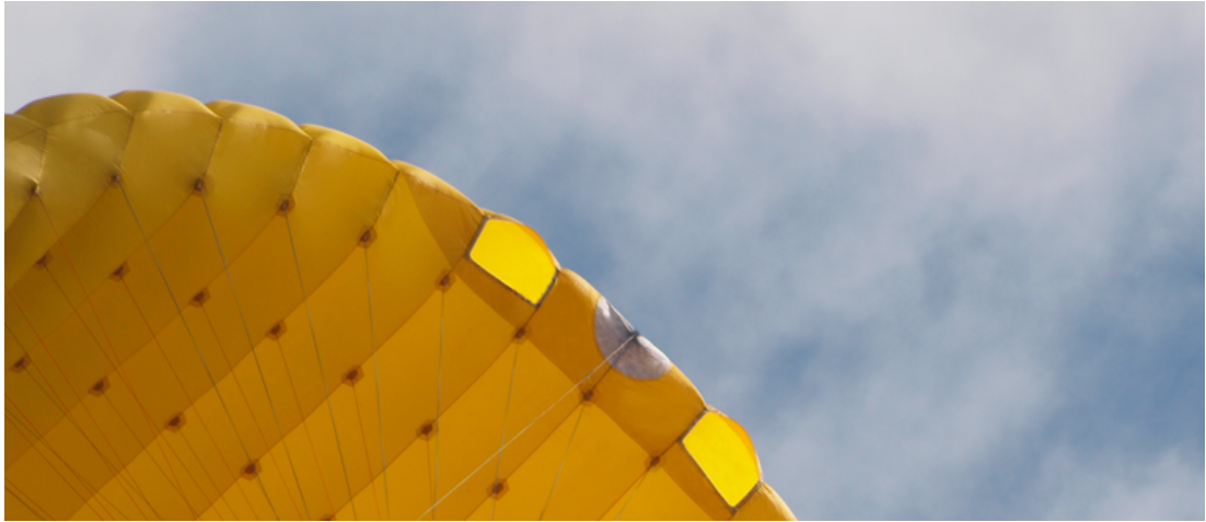
Figure 3.3: Ram air kite details - Two holes in the leading edge keep internal pressure higher when flying. Some cables composing the bridle system are also visible. Picture from (13).
