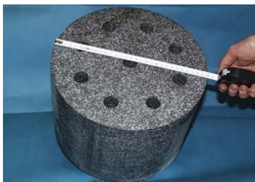
Figure 3.10: Storage made of PCM and compressed graphite[45].
