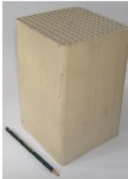
Figure 4.5: Storage unit used at the Jülich solar plant[64].
