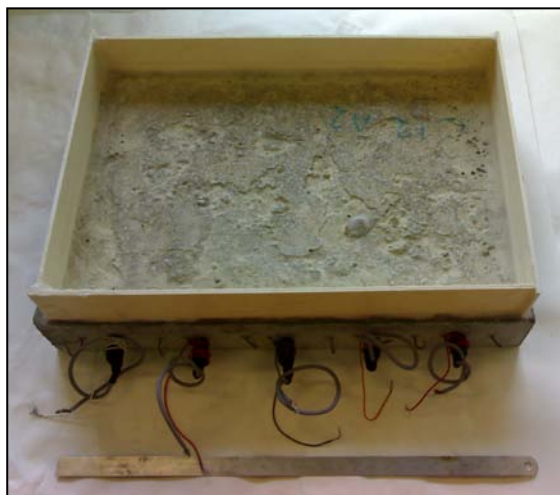
Figure 4. 6: Condition of exposure of the samples (ponding)
