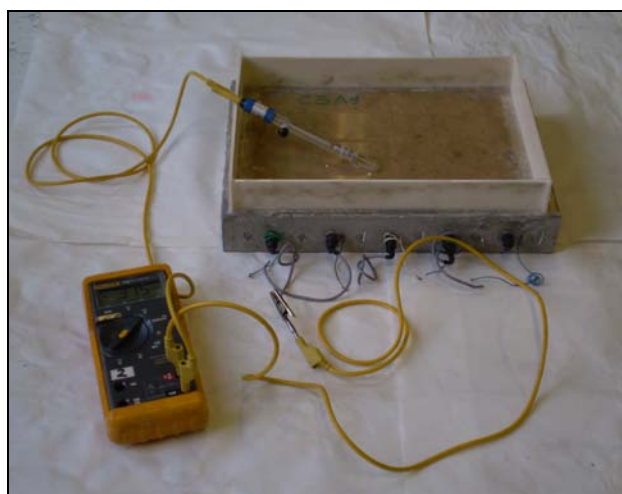
Figure 4. 7: Tools for measuring the corrosion potential
