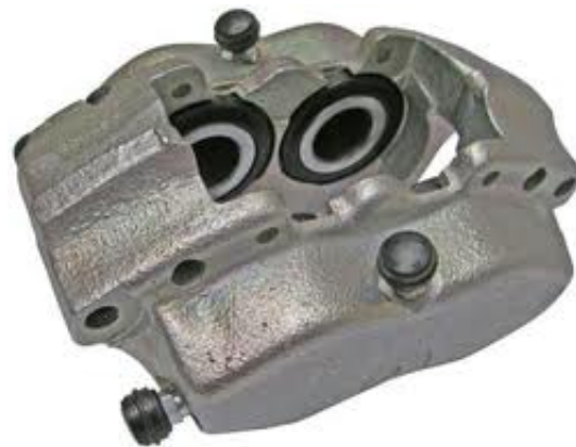
Figure 1.5: Fixed Caliper with Four Pistons
