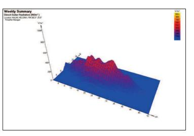
Figure 5.11 Direct Solar Radiation in Malmi, Helsinki
