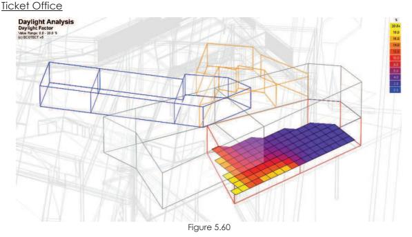
Average value of DLF = 8.0%, Min value of DLF = 2.0%, Max value of DLF = 20.0%The ticket office has large scale of glazing on the west facade and half of the south facade. Considering the high value of daylight factor (20%), automatic curtains system is also proposed to be installed on the inner side of glazing.
