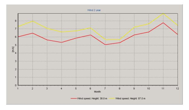
Fig 4.6 Graph showing the mean wind speed at the heights 38 m (red) and 87 m (yellow).
