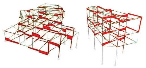
Fig 4.22 3D view of shear force diagram of frames in SAP2000
