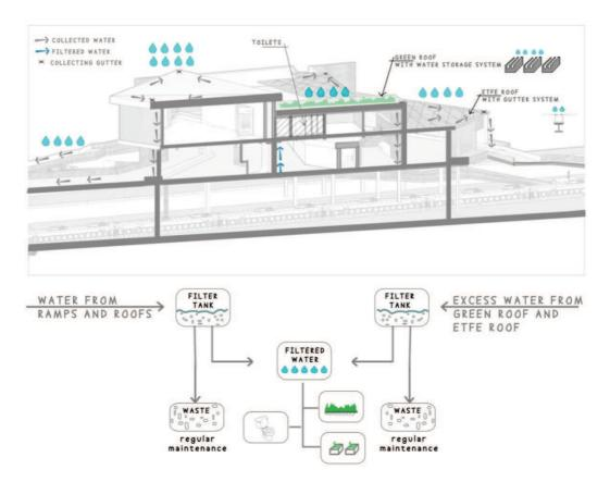
Figure 5.66 Schematic diagrams for rain collection system
