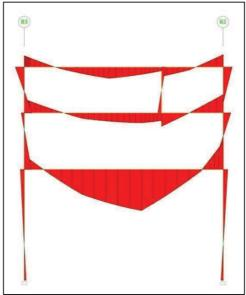
Fig 4.20BM diagram of semi-open platform on Axis BE (KN/M/C)
