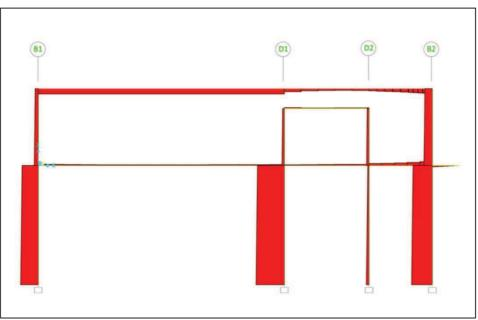
Fig 4.29AF diagram of multifunctional building on Axis BA (KN/M/C)
