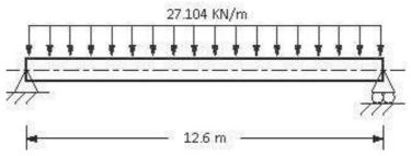
In calculation, we rougly conside it as simply supported beam,  $Md = qL^2 / 8 = 27.104 \times 12.6^2 / 8 = 537.88 \text{ KN} \cdot \text{m}$
