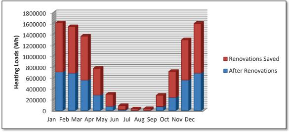
Comparing to loads 129260 W/  $M^2 \cdot a$  before renovations, the heating loads in Zone Services has dropped to 52560 W/  $M^2 \cdot a$ . The **59.3%** of heating loads are saved after renovations.
