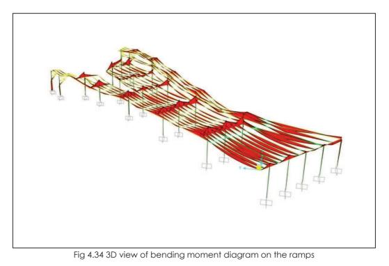
According to the simulated result obtained from the SAP2000, the structure of ramps is satisfied by assessments.
