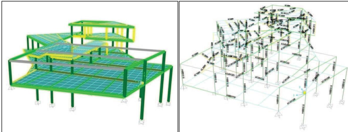
Fig 4.8 Simulated structural model of The semi-open platform in SAP2000
