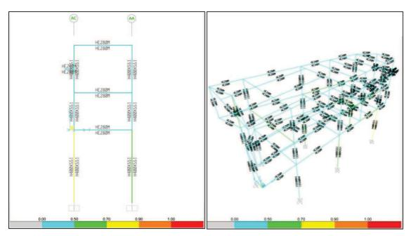
Frame on axisA5 (for most frames,stress limit ratio is below 0.50, for two columns on the ground floor, it is between 0.50 and 0.90)
