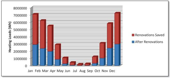
Comparing to loads 129260 W/  $M^2 \cdot a$  before renovations, the heating loads in Zone Services has dropped to 52560 W/  $M^2$ . a. The **59.3%** of heating loads are saved after renovations.
