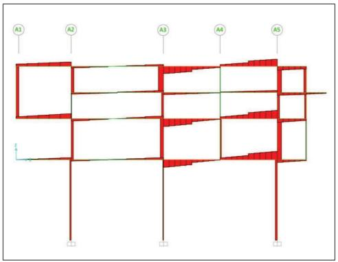
Fig 4.23 SF diagram of multifunctional building on Axis AC (KN/M/C)
