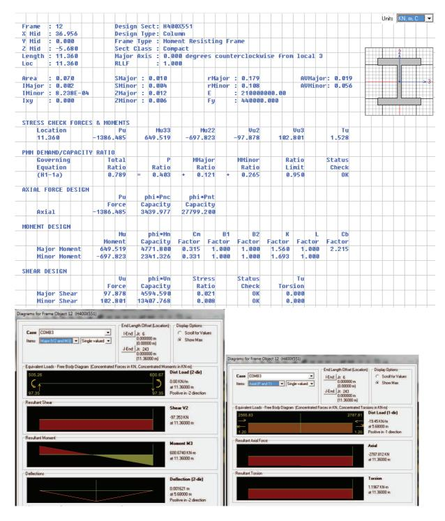
N<sub>Ed</sub> = 2787.81 KN M<sub>Ed</sub> =600.67KN ·m V<sub>Ed</sub> = 97.35 KN
