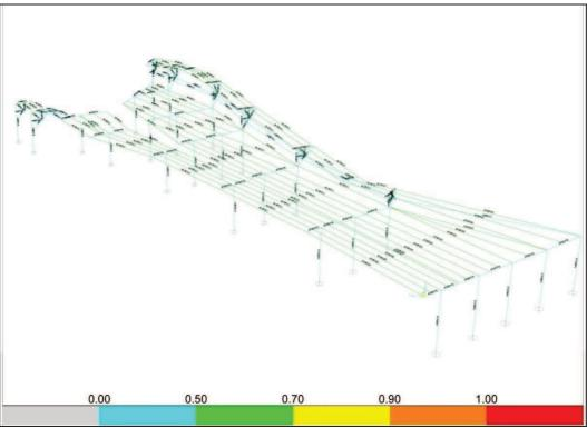
Fig 4.33 3D view of stress limit ratio on the ramps.
