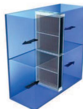
Figure 5.29 Airstreams through heat pipes
