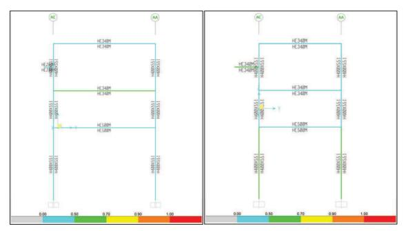
Frame on axisA2 (for most frames,stress limit ratio is below 0.50, for the beam on the second floor, it is between 0.50 and 0.70)
