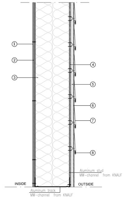
(1) Acrylic bonded water based exterior façade paint
