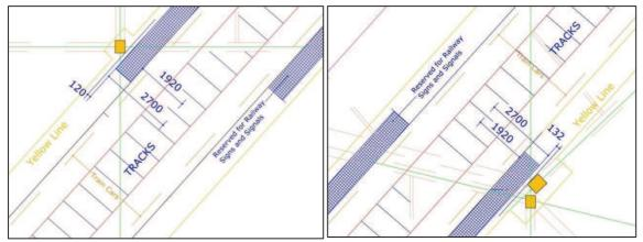
Fig 4.3 .1 Clearances beside A3AC column Fig 4.3 .2 Clearances beside A5AA column
