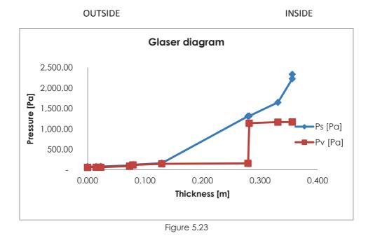
Due to saturated pressure is more than vapor pressure for every layer, there is no condensation risk in the roof T\_07\_01.
