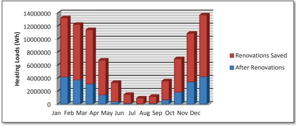
Comparing to loads 286810 W/  $M^2$  a before renovations, the heating loads in Zone Foyer has dropped to 77999 W/  $M^2$  a. The **72.8%** of heating loads are saved after renovations.
