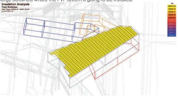
Figure 5.65 Solar exposure analysis for MPU roof
