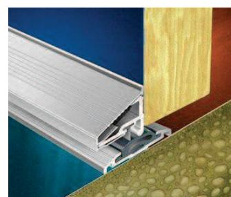
Figure 5.28 Air barrier at the window frame
