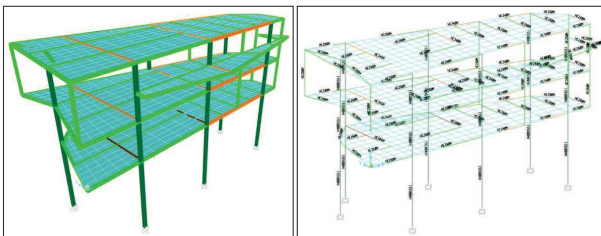
Fig 4.7 Simulated Structural model of multifunctional building in SAP2000
