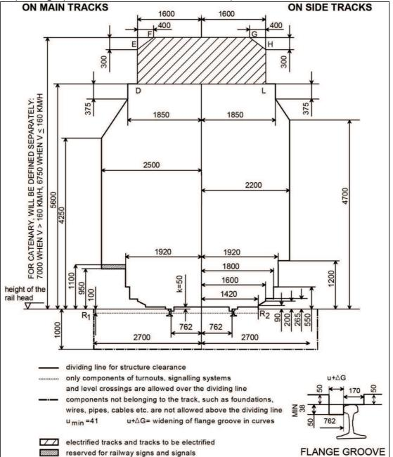
Fig 4.2 Principal dimensions of the structure gauge in Finland
