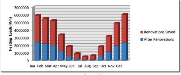
Comparing to loads 183952 W/ $M^2$  a before renovations, the heating loads in Zone MPU has dropped to 69522 W/ $M^2$  a. The **62.2%** of heating loads are saved after renovations.
