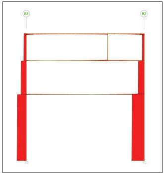
Fig 4.28AF diagram of multifunctional building on Axis BE (KN/M/C)
