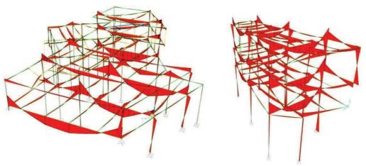
Fig 4.18 3D view of bending moment diagram of frames in SAP2000
