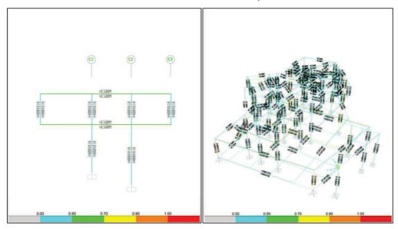
Frame on axisCA (for columns, stress limit ratio is below 0.50, for beams, it is between 0.50 and 0.90)
