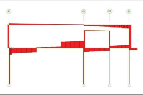
Fig 4.25 SF diagram of semi-open platform on Axis BA (KN/M/C)
