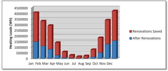
Comparing to loads 236119 W/  $M^2$  a before renovations, the heating loads in Zone Seating Area has dropped to 75390 W/  $M^2$  a. The **68.1%** of heating loads are saved after renovations.
