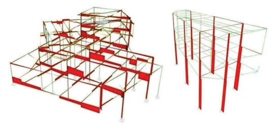
Fig 4.26 3D view of axial force diagram of frames in SAP2000
