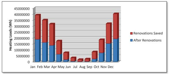
For the total heating loads in all visible zones, the heating loads drops from 163636 W/ $M^{2}$ .a to 70966 W/ $M^{2}$ .a. Generally, the **56.6%** of energy has been reduced. In the mean while, we have achieved the goal that the energy on space heating should not exceed the value 56-84 kW/ $M^{2}$ .a (solution value: **70.966 kW/M^{2}**.a)- a national standard of Finland for the low energy buildings according to National Building Code of Finland.
