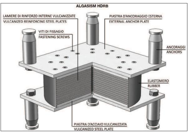
Fig 4.14 High Damping Rubber Bearings / Lead Rubber Bearings
