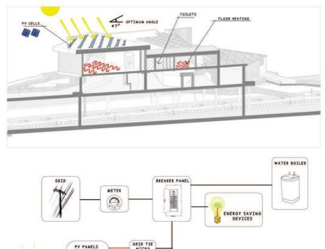
Figure 5.64 Schematic for PV system-grid connection
