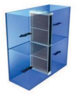
Figure 5.29 Airstreams through heat pipes
