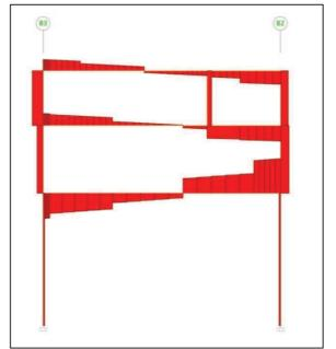
Fig 4.24 SF diagram of semi-open platform on Axis BE (KN/M/C)
