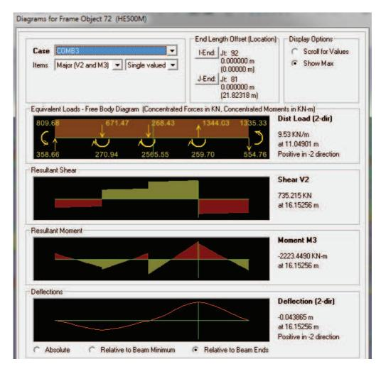
M<sub>Ed</sub> = 2223.45KN ⋅m V<sub>Ed</sub> = 735.22 KN HE 500 M wide flange section is selected.
