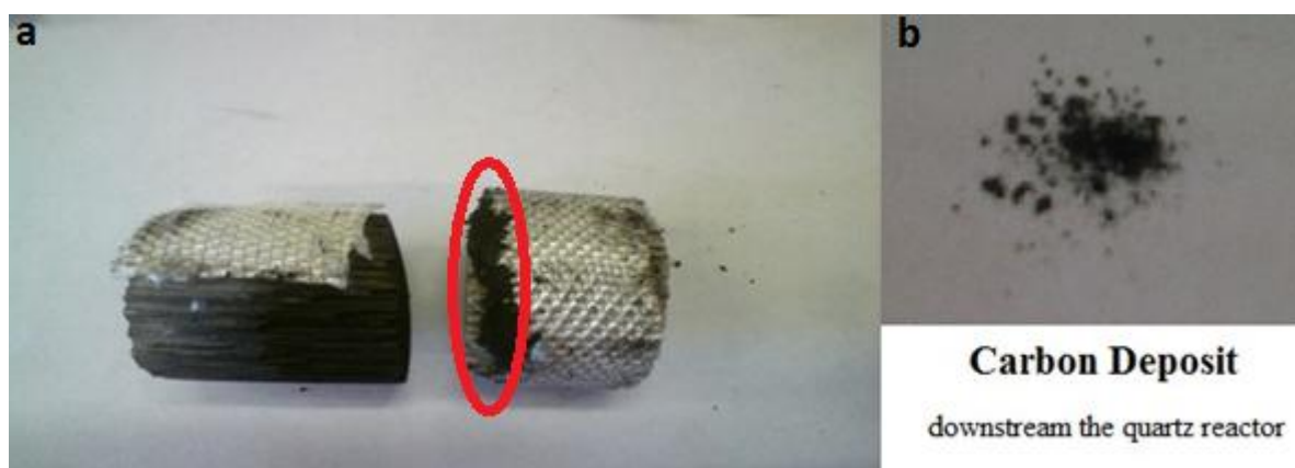
Figure 7.1: Typical carbon deposition after a C_3H_8 test at 4 bar for 7 hours. Panel a: catalyst on the left, Back Heat Shield on the right; panel b carbon deposit collected on the flange surface.
