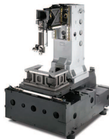
FIGURE 2.2: Frame of a machine tool [Sod12]
