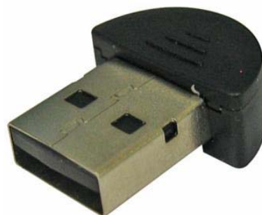
Figure 3.24 - Nano Bluetooth USB 2.0 dongle by Mediacom
