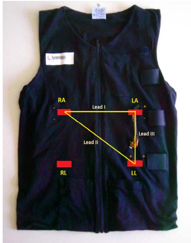
Figure 3.8 - T-shirt with the Einthoven triangle and its lead: Lead I: LA - RA , Lead II: LL - RA , Lead III: LL - LA .
