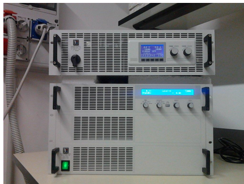
Figure 4.1 Test equipment: a controlled DC source EA-PSI 8240-170 and a controlled electronic load EA-EL 9400-150. The equipment is controlled via interface cards with a control program written in Labview environment.
