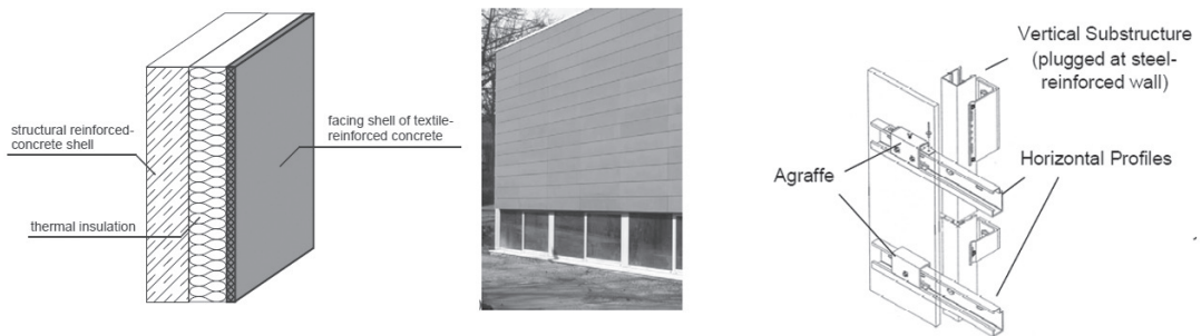
Figure 3.81: Sandwich panel used for curtain wall, Aachen University
