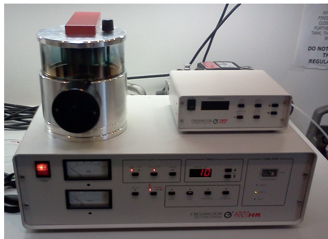
Figure 25 cressintong sputter for gold deposition
