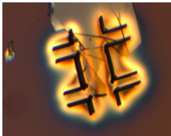
Figure 40 pattern transfer on a graphene flake without a protective membrane. A small misalignment is visible. Furthermore an halo on the border of the milled area is indicating a possible local contamination
