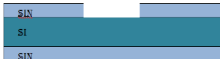
Figure 19 schematic drawing of the sample after RIE etching and resist removal
