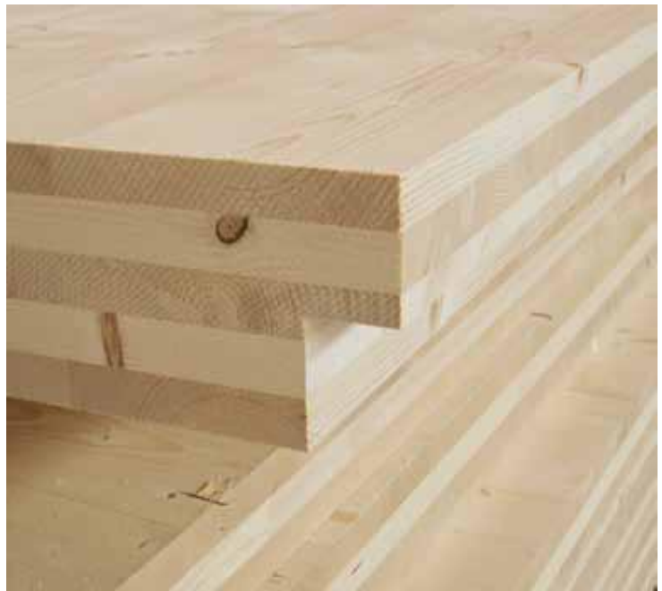
Figure 5.1. Cross laminated timber
