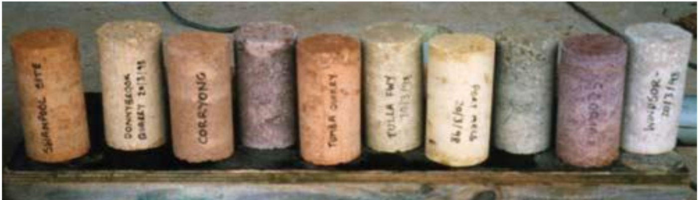
Fig. 6.23 Stabilized Rammed Earth samples made from different colored earths
