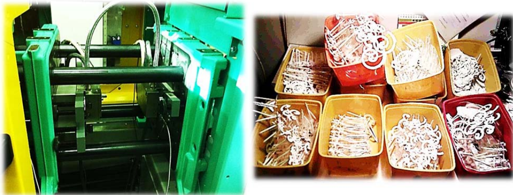
Fig. 102 Mould mounted on the machine and cataloged results for the spiral component
