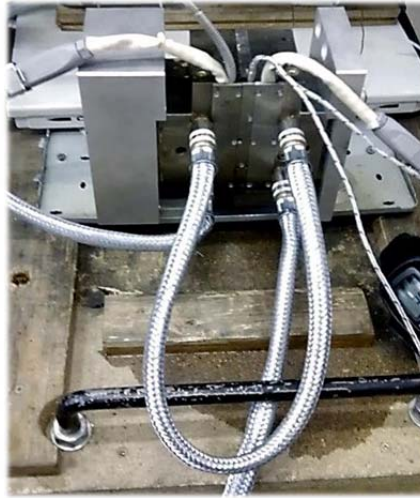
Fig. 97 Mould with cable connection for thermal experiment
