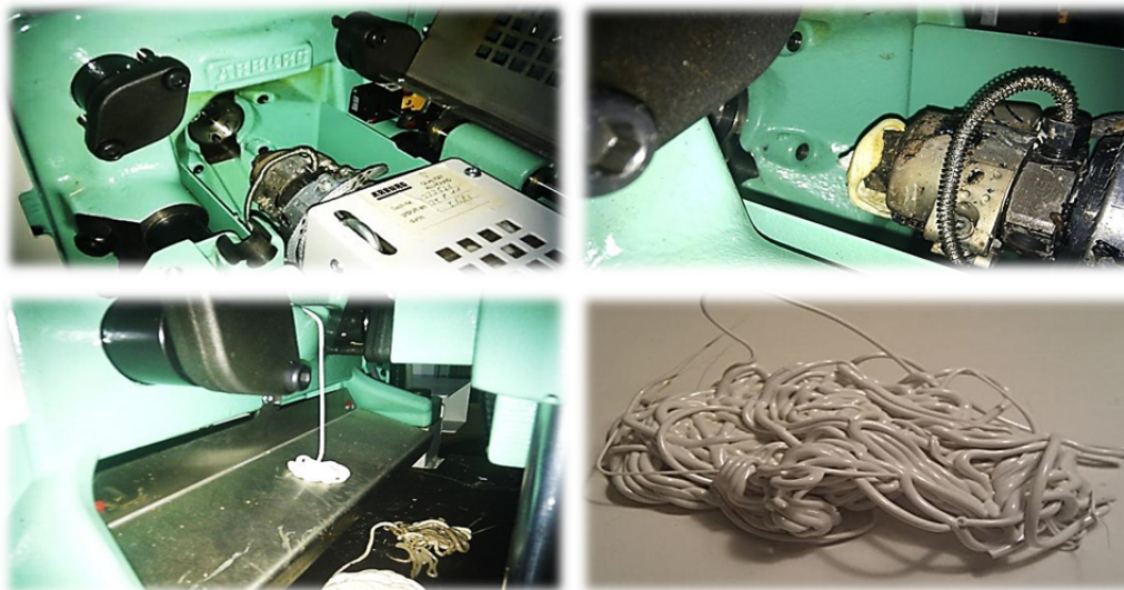
Fig. 157 Nozzle cleaning by using polypropylene
