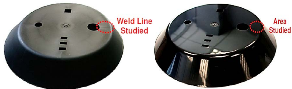
Fig. 35 Weld line studied on ABS polymer at Swansea University for GIWW Ltd
