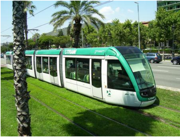
Figure 207 Barcelona Grass lined Tramway
