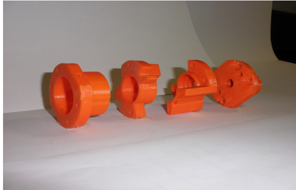
Figure 7: optical groups realized with a 3D printer.
