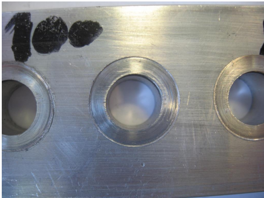
Figure 2.3 the area on the clamped component contact with under bolt head
