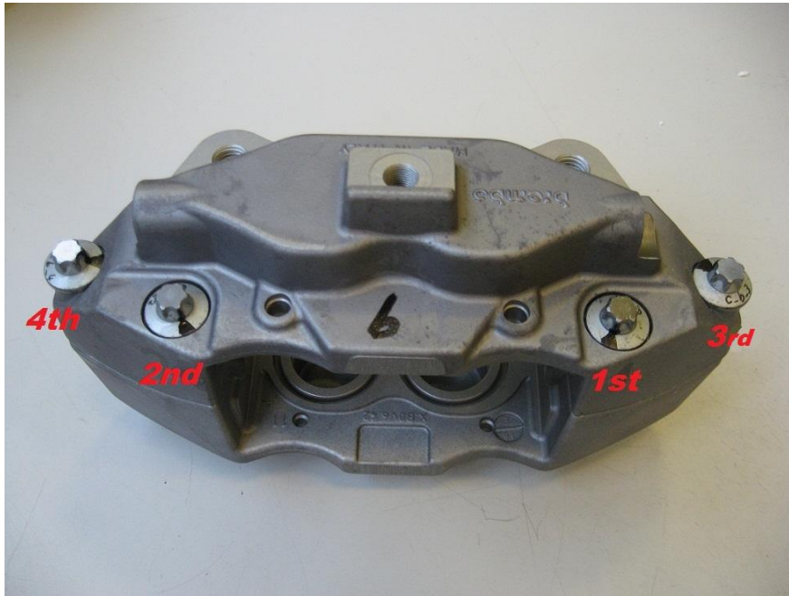
Figure 5.19: tightening sequence of the caliper's bolts
