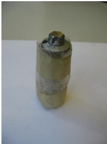
Figure 4.8: The reference bolt protected by PE bubble paper
