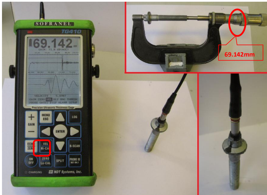
Figure 4.16: Velocity calibration of ultrasonic device.
