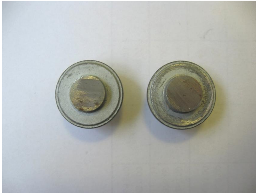
Figure 2.2 The bolt under head surface of before(left)/after(right) tightening
