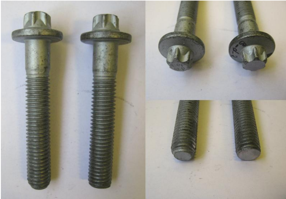
Figure 4.2: A comparison between original bolt (left) and flattened bolt (right)
