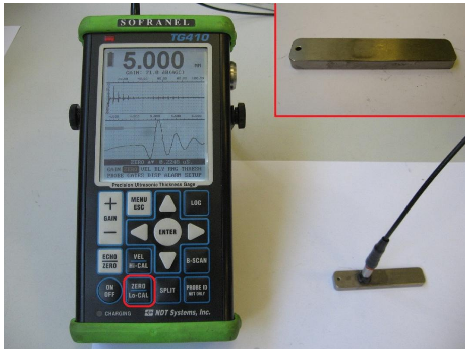
Figure 4.15: Zero calibration of ultrasonic device and the reference sample.
