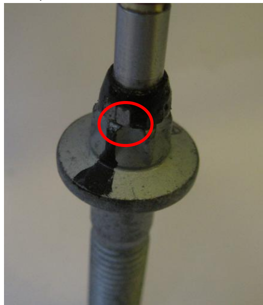
Figure 5.3: the mark signed on ultrasonic sensor and bolt head
