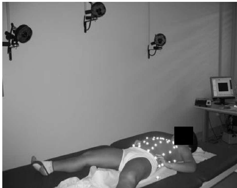
Figure 4.1: Experimental set-up for the analysis of chest wall volumes in supine position via opto-electronic plethysmography in a DMD patient
