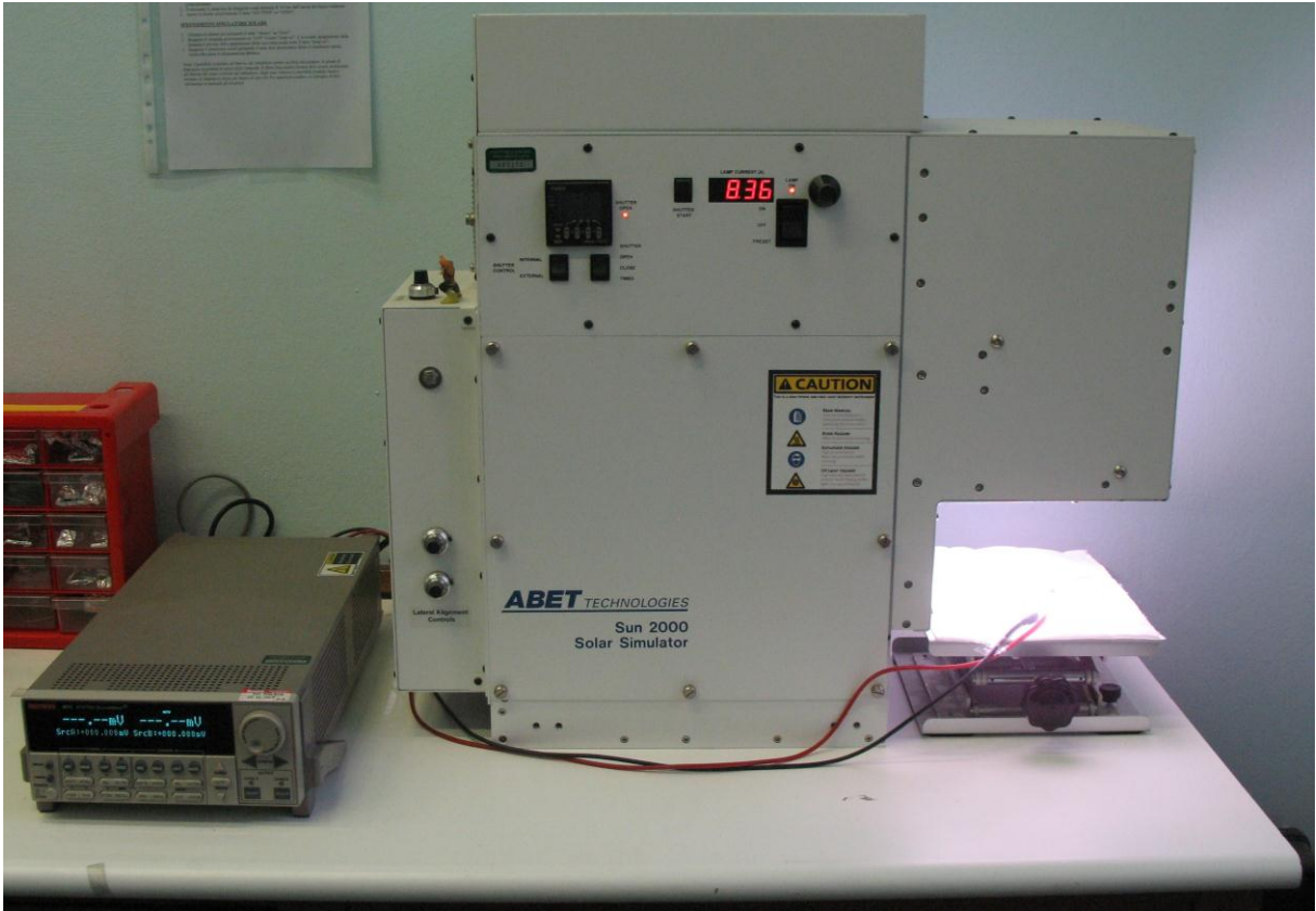
Figure III.11 The Keithley 2612 Digital Multimeter is reported on the left while the Sun 2000 Solar Simulator on the right.
