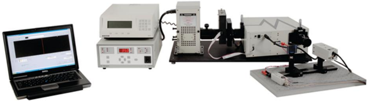
Figure III.14 Set up of the instrument used to perform EQE tests.
