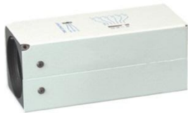
Figure III.15 Silicon detector used in performing EQE test.
