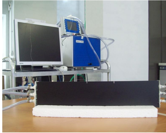
Figure 4.3: Thermostatic bath linked to the black sample.
