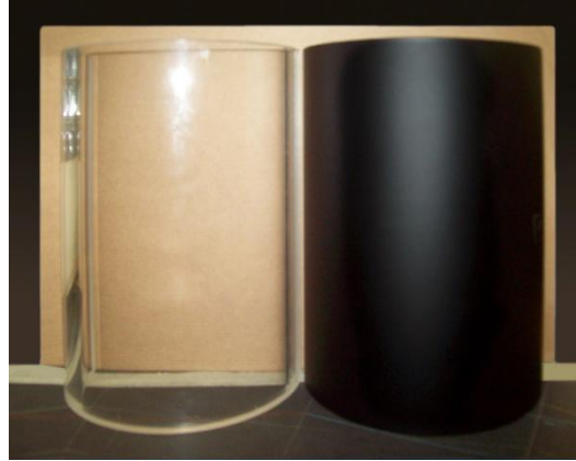
Figure C.3: Cylindrical sample, before and after the coating.
