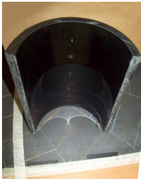
Figure C.4: Flaws on the cylindrical sample.
