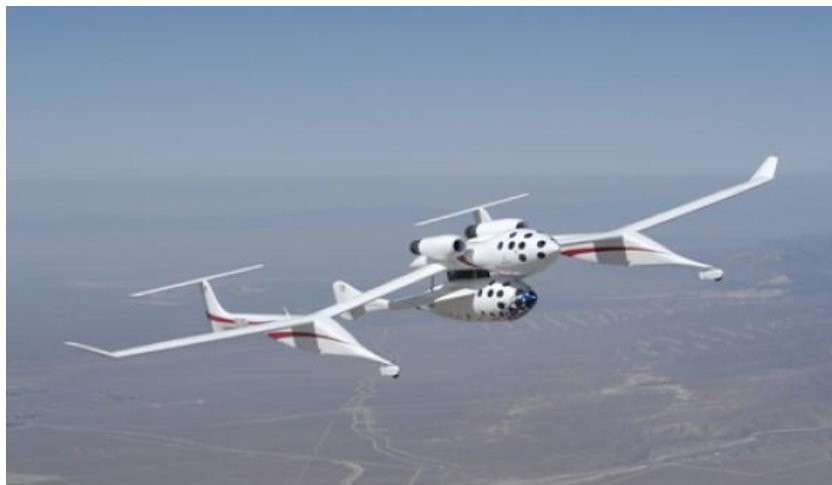
Figure 2.10: Space Ship One carried aloft by the White Knight [Credit: Scaled Composites, LLC].
