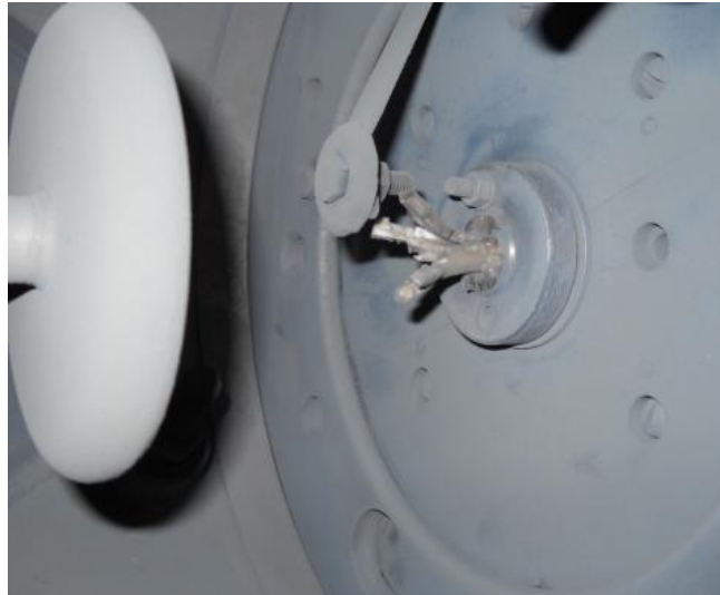
Figure 4.3: UDP-5 wire support broken by shockwaves generated by wire explosion.
