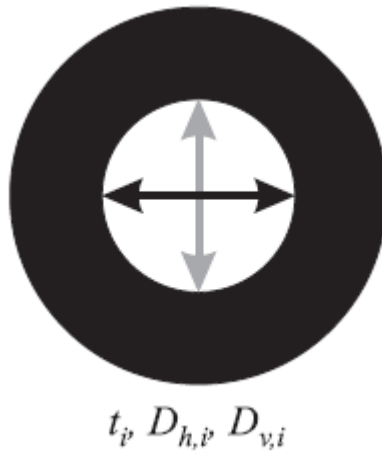
Figure 6.7: Time-resolved quasi-steady regression rate: definition of mean sampled diameter [75].
