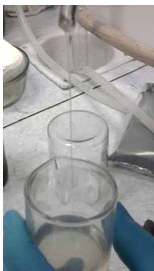
Figure 4.10: Homogeneous solution of FLUOREL and Ethylene acetate.
