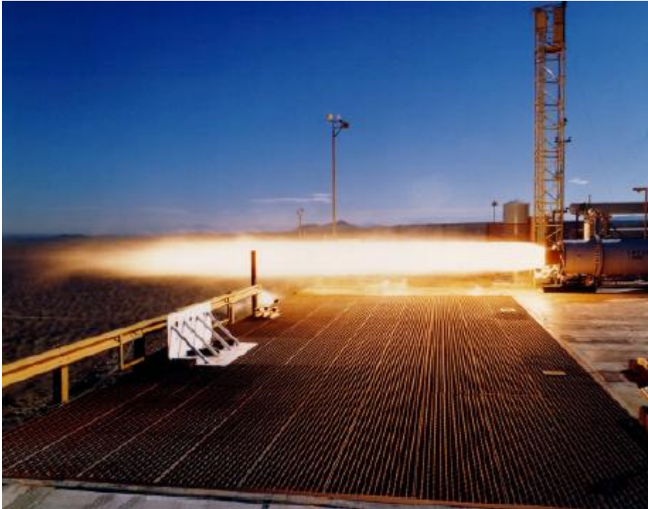
Figure 2.8: Test of AMROC H-500 motor, using LOX/HTPB propellant [5].
