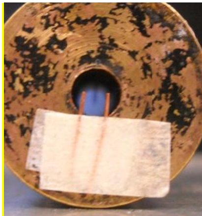
Figure 6.4: Sight cylinder used for sample alignment
