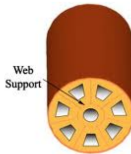
Figure 2.9: High burning multiport surface geometry
