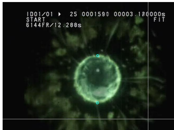
Figure 6.8: Example of Vertical diameter sampling, note head-end burning.
