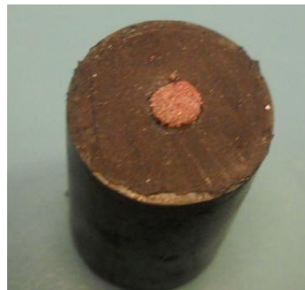
Figure 6.5: HTPB+ 10% Cu sample with pyrotechnical charge.
