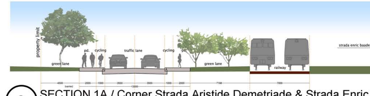
2 SECTION 1A / Corner Strada Aristide Demetriade & Strada Enric Baader NTS PROPOSED SITUATION
