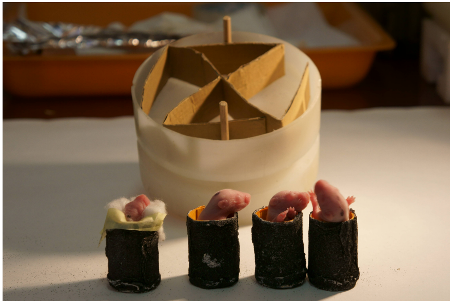
Figure 5.2: Picture of mice in borated paper cylinders, with the polyethylene irradiation container in the back
