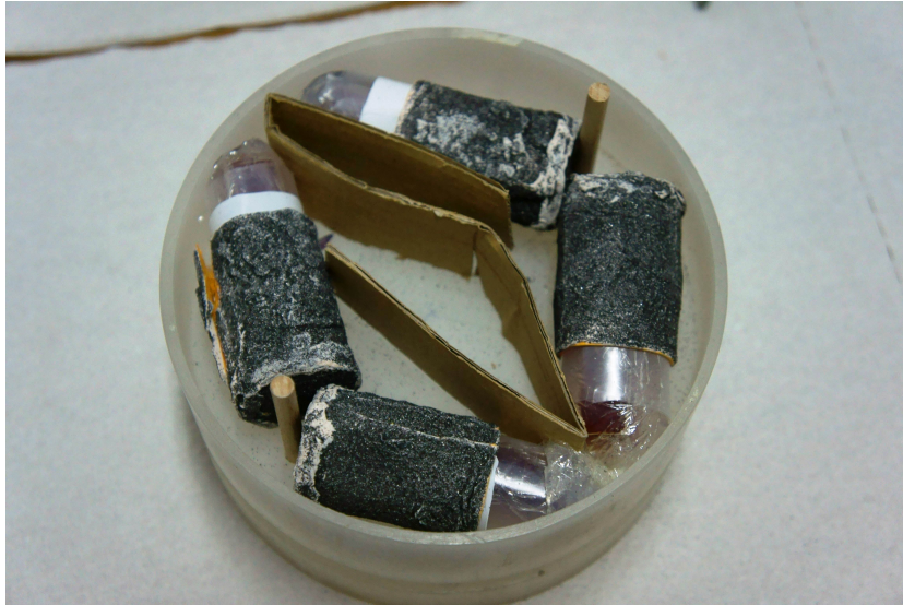
Figure 5.16: Photo of cuvette dosimeters in mice phantoms, with shielding
