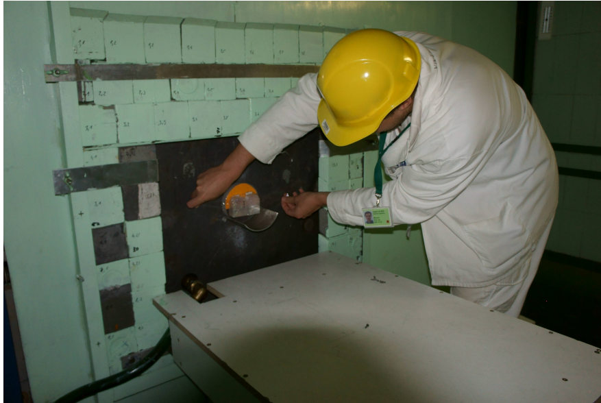
Figure 5.3: How the irradiation container was positioned towards the beam
