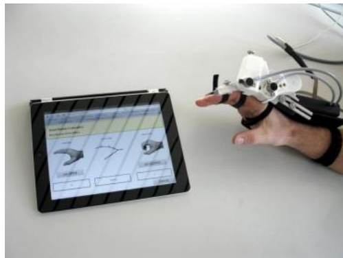
Fig.2.12: robotic hand orthosis during calibration procedure.
