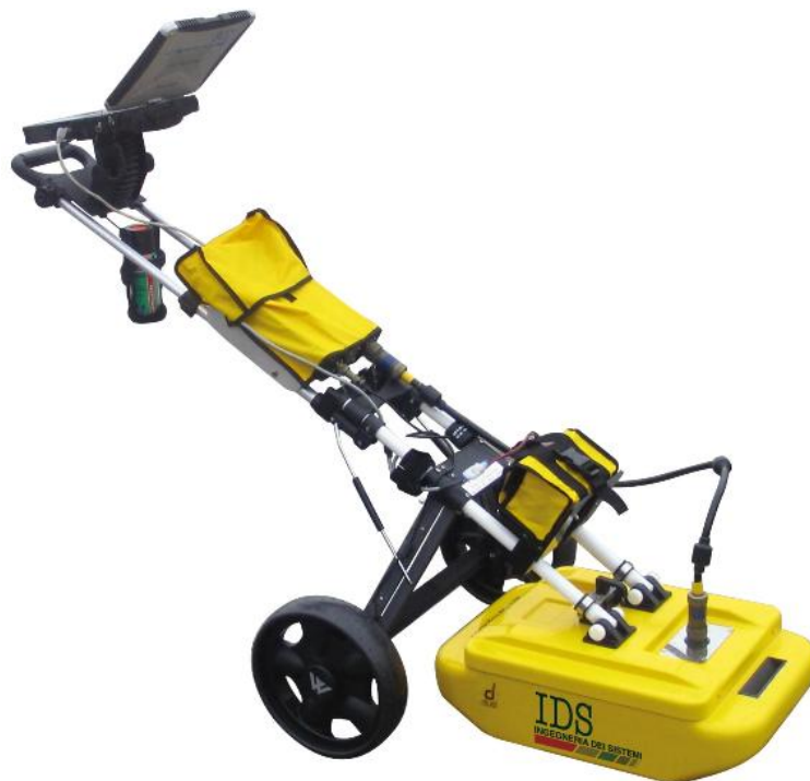
Figure (29): Detector Duo GPR device used in acquisition.
