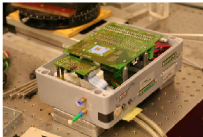
Fig 4.3 complete image of the apparatus of the detector consists of a motherboard suspended on four supports, by a tab switching to switch from the phase drift to that of integration, and by a tab host preamplifiers voltage.
