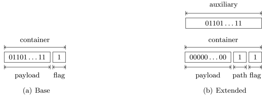
Figure 3.5: Layout of the container type. In the base version only one bit is needed to encode the barrier state, all others can be used to pack partial reduction values. The extended layout uses one more bit to find whether the reduction partial value is packed into the container payload or stored in the auxiliary variable
