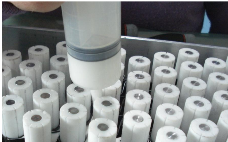
Figure 6.6 – The application of silicon rubber by a syringe
