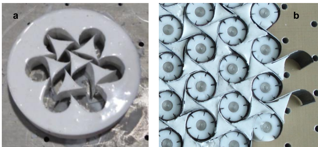
Figure 6.7 – (a) Triangular shaped rubber inserts inside the silicon dam (b) Assembly of rubber inserts on the rib mold
