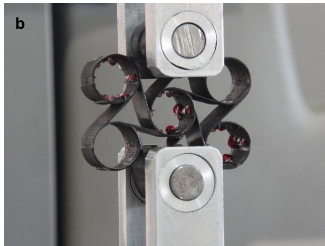
Figure 4.13 – Chiral unit cells under tension – compression testing (a) GFRP chiral unit (b) CFRP chiral unit
