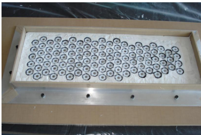
Figure 6.8 – Complete chiral rib with all 5 – ply ligaments
