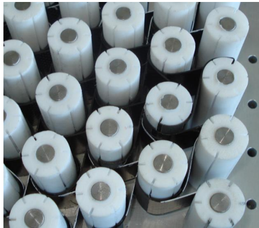
Figure 6.5 – Implementation of silicon rubber inserts; Silicon rubber inserts not injected yet
