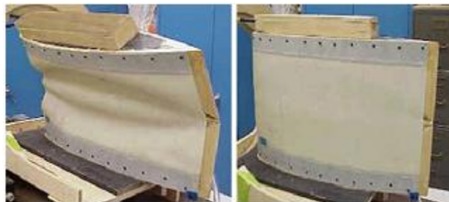
Figure 2.9 – Morphing wing covered with SMP skin on a test jig
