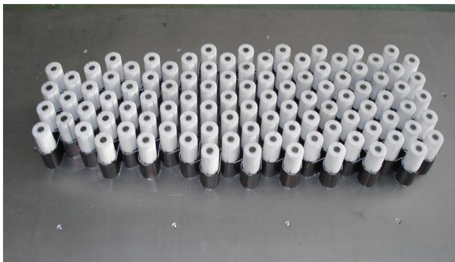
Figure 6.2 – Teflon – made cylinders on the assembly mold
